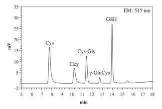
Fig. 2. Chromatogram of mixture of thiols in optimized conditions described in the section *Chromatography*
